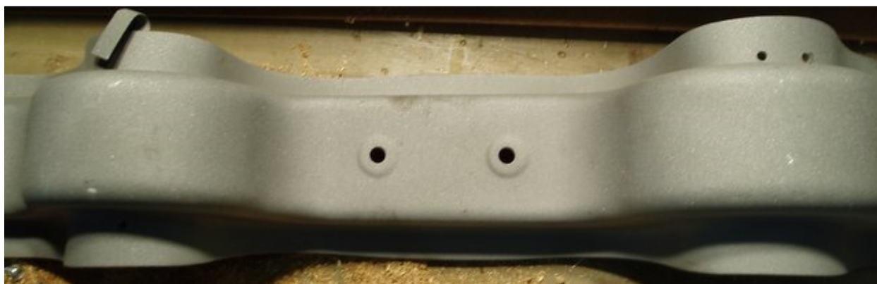
Rear Cross member after sand blasting.
