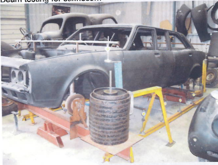
Beam testing for stiffness...
