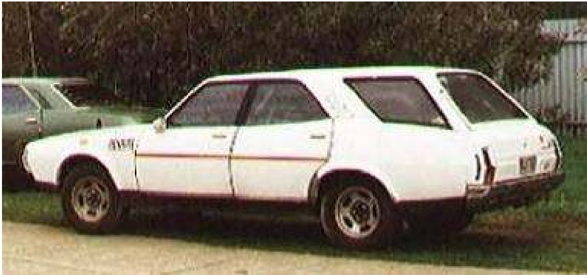
Replica Two – jacked up suspension with off-road wheels and tyres.
