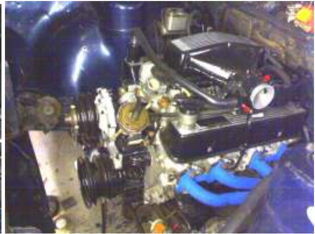
4.6 drops straight in on P76 engine mounts
